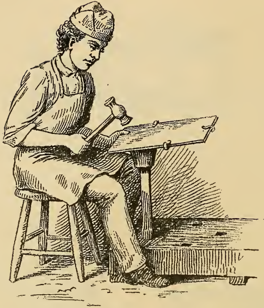
Fig. 19.—Planishing at the Block.
